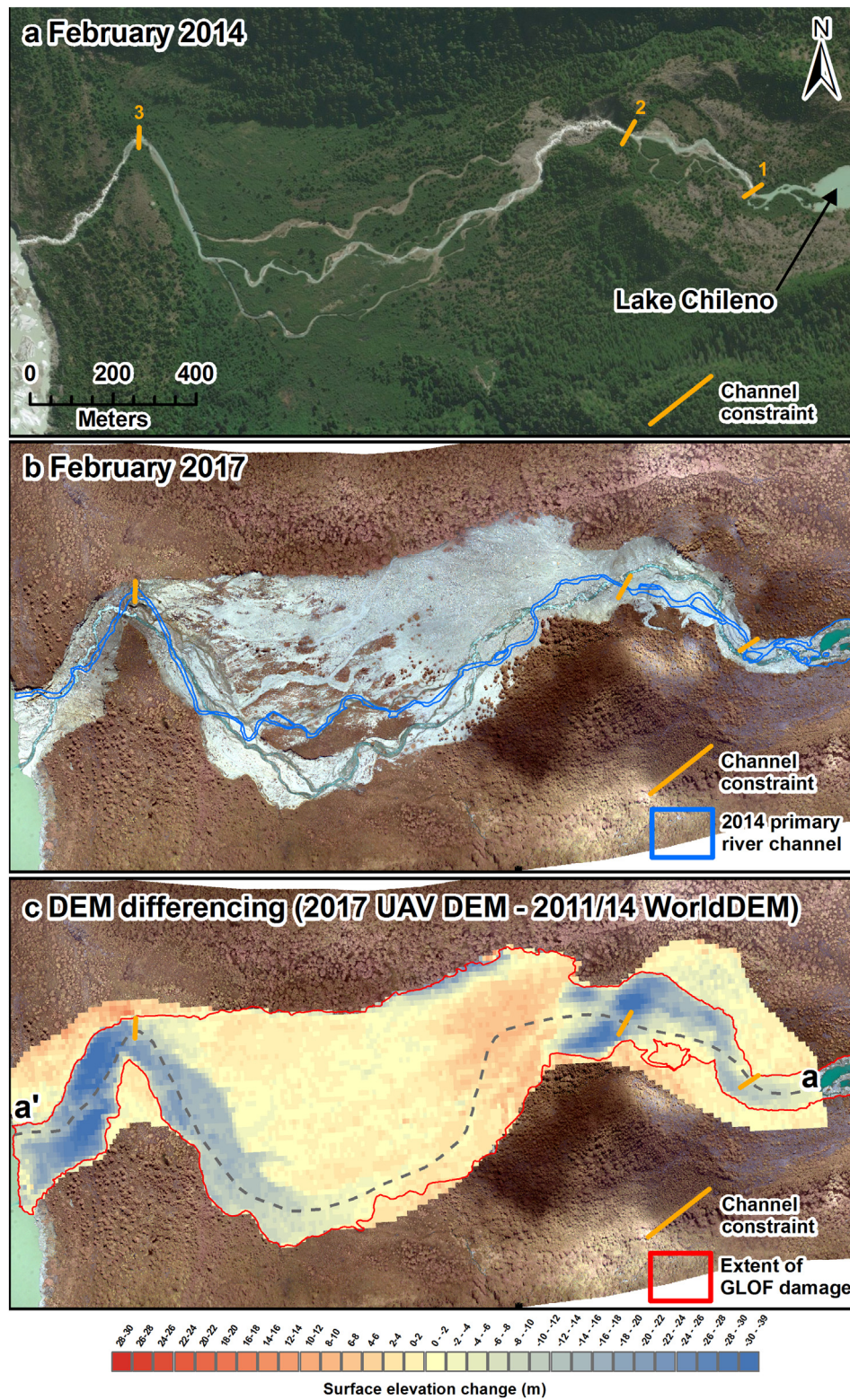
Fig. 4. Geomorphology of the Chileno Valley before (a) and after (b) the GLOF event that occurred in December 2015. Post-GLOF surface elevation changes are shown in image (c).
